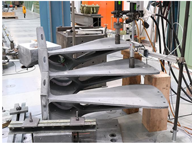
Fig. 4—Steps assembled with SMA (Empa, CH).
